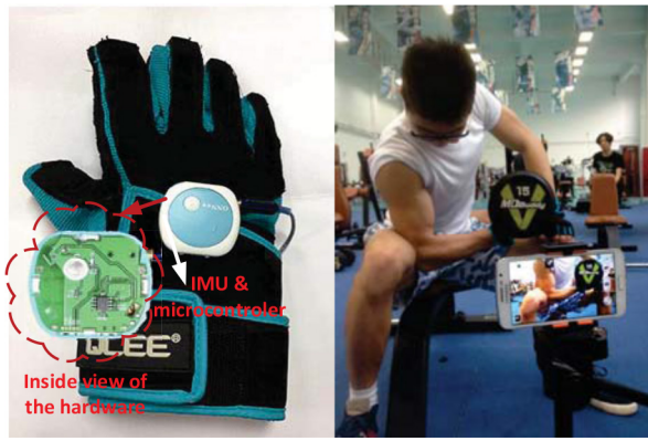
Fig. 1. Left: The present prototype of iCoach. Right: Experimental scenarios. iCoach is a smart device and application that monitors exercise activities and provides feedback in real time. It can be seamlessly embedded with fitness glove and thus is nearly unobtrusively. We conduct experiments in a university gym to evaluate its performance.
