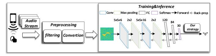
Figure 3: The data processing workflow of MetaDigit
