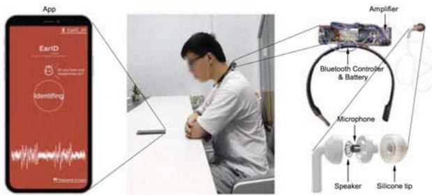
Fig. 5. The hardware and software of EarID system.
