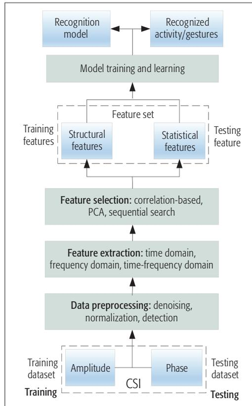
Figure 4. The general architecture of data-driven Wi-Fi radar.
